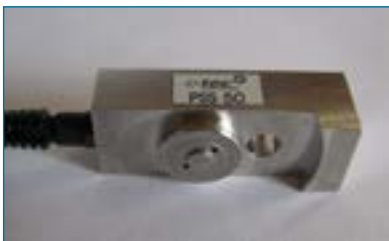
Piezoelectric quartzsensor for installation at the press frame
