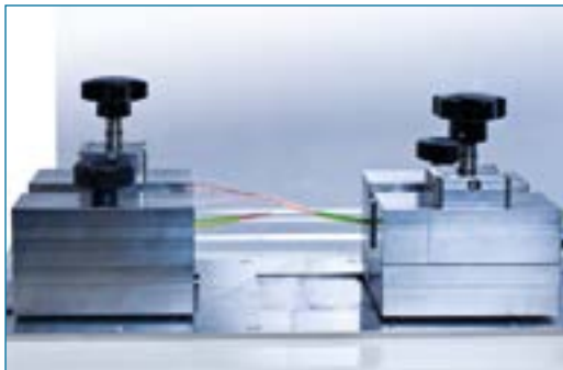
Universal clamping jaws for different sizes of crimps, e.g. break behaviour of a cable with \text{Ø } 0.75\text{mm}^2
