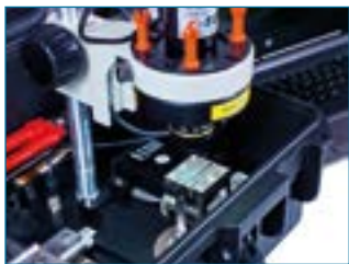
Powerful measuring microscope with 4x zoom
