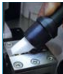
Fine polishing of the crimp
