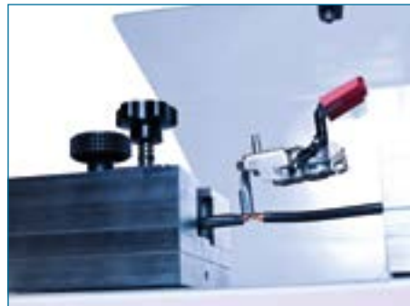
Testing of cables with a larger diameter, e.g. pull force measuring of a battery terminal crimp
