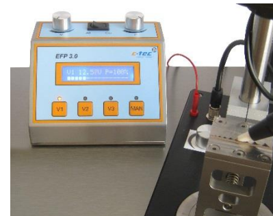
Electronic fine polishing of a crimp cross section
