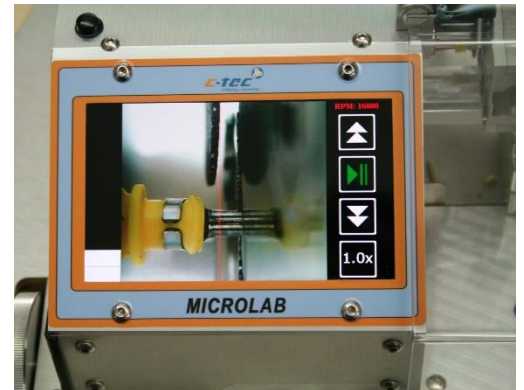
Cut control with an optional Visual Cut Camera (VCS)
