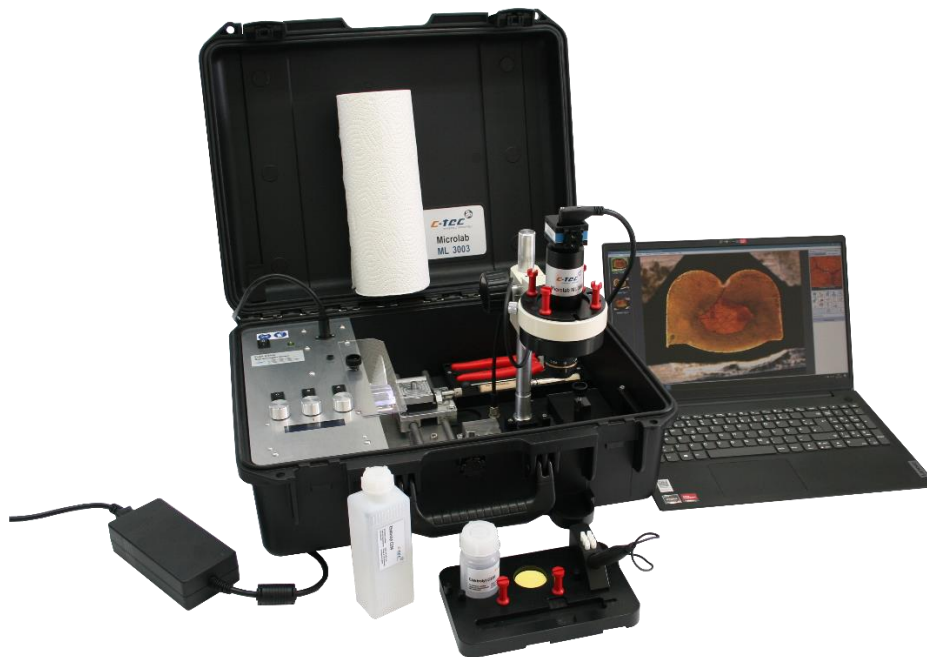
Microlab ML 3003 in operation (standard delivery without notebook)
